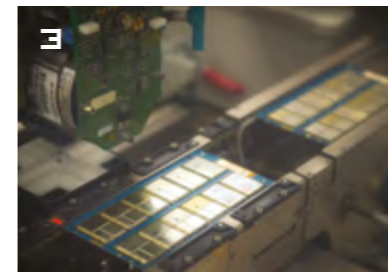
1 State-of-the-art pick-and-place equipment
